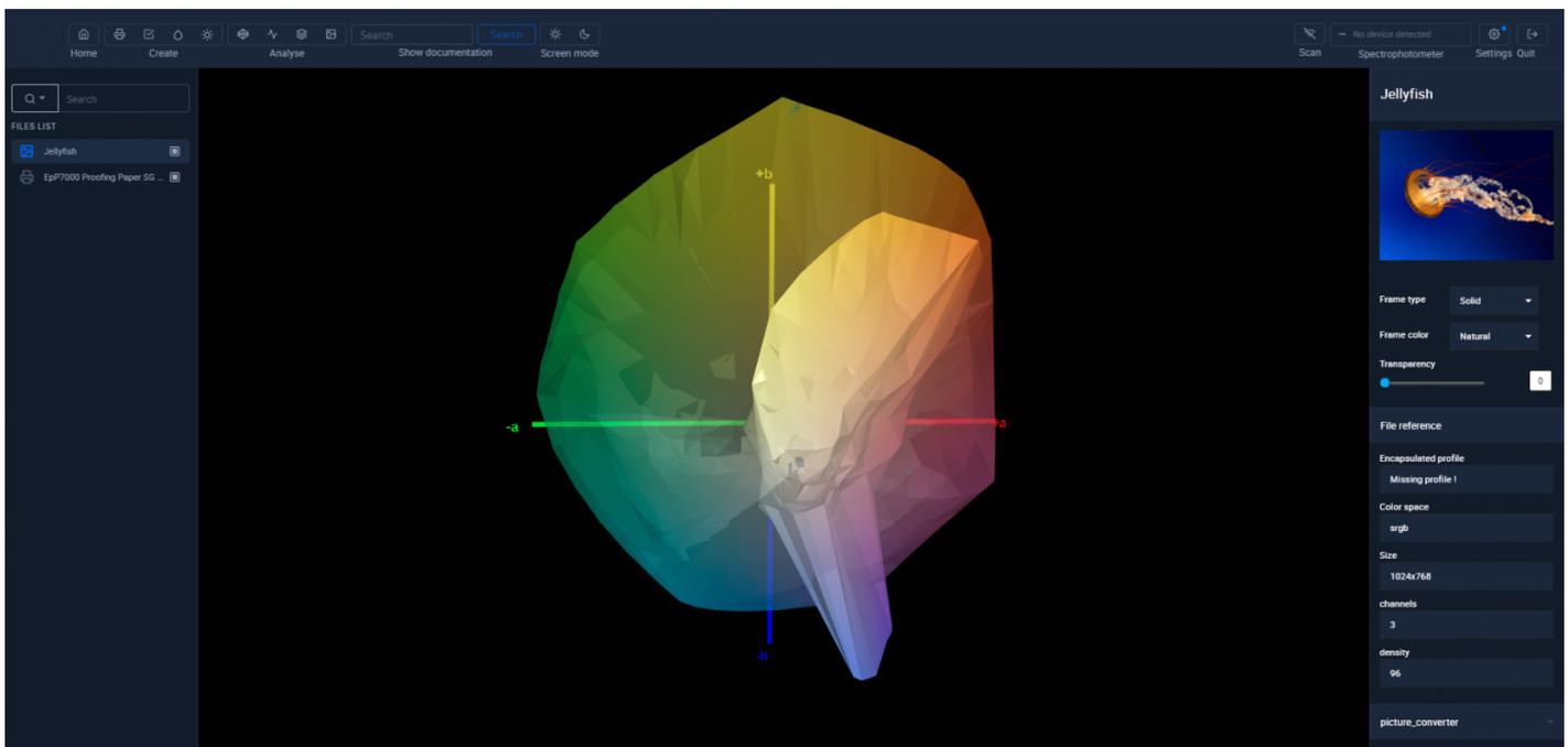
In this example we can see by superimposing the two gamuts, that the saturated blue of the jellyfish image comes out of the reproducible color gamut of the printer.
