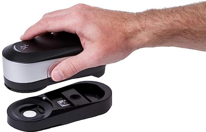
Make sure that the white calibration ceramic is not covered by the protection
