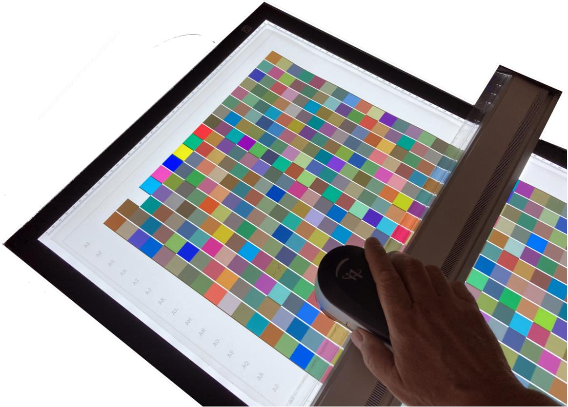
The cadence must be slower than for measuring a target measured in reflective mode.
